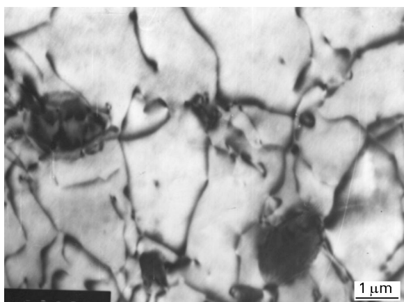
Figure 15 Transmission electron micrograph of alloy 2 in the quenched condition.
